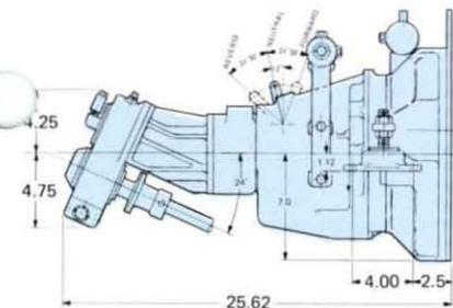
**WARNER Hydraulic Vee-Drive.** A Warner gear coupled to a Walter vee-drive. Ratios of 1.29:1, 1.67:1, and 2:1. Weight 135 lbs. Turns left hand propeller.
