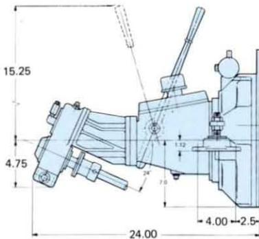
**PARAGON SAOV.** Use our front end exhaust outlet with this manual vee-drive. Available in ratios of 1.29:1, 1.67:1 and 2:1. Weight 90 lb. Turns left hand propeller.
