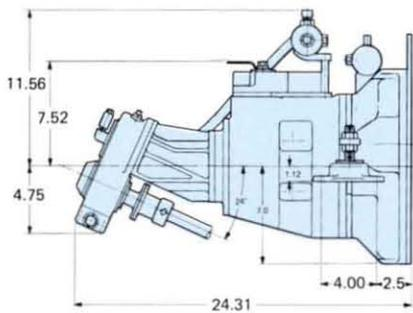
**PARAGON Hydraulic Vee-Drive.** A Paragon P20 hydraulic gear close-coupled to a Walter vee-drive. Ratios of 1.29:1, 1.67:1, and 2:1. Weight 132 lb. Turns left hand propeller.
