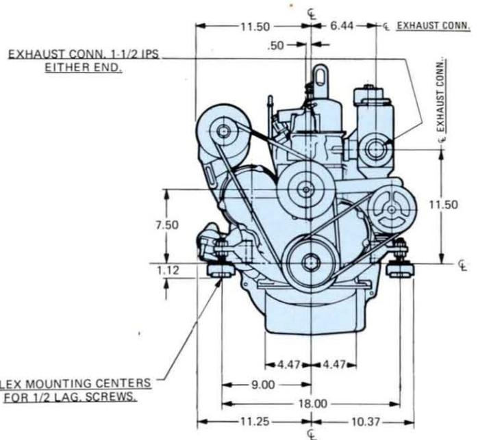
**WESTERBEKE Short Profile Sailing Gear.** The most compact 2:1 reduction package ever! Features positive neutral for free-wheeling, silent-running shaved case-hardened helical gears, heavy-duty tapered roller bearings, and instant acting fingertip control. (Use Morse 33C cable or equal.) Weight 25 lbs. Turns right hand propeller. Drawing above shows Walter vee-drive close coupled to the sailing gear. Reduction, 2:1. Weight 70 lbs. Turns right hand propeller.
